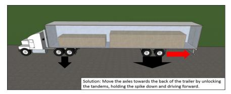
**Caution!** – There are rules governing how far back tandems can be placed. **California has a "Bridge Law" which states that the center of the rear tandem axle hub can be no more than 40 feet back from the kingpin on a 53 Ft trailer.** Most 53 Foot trailers are marked at the "40 Foot" mark. **\*\*Check your local state restrictions for guidance, it is your responsibility to comply with laws\*\***
